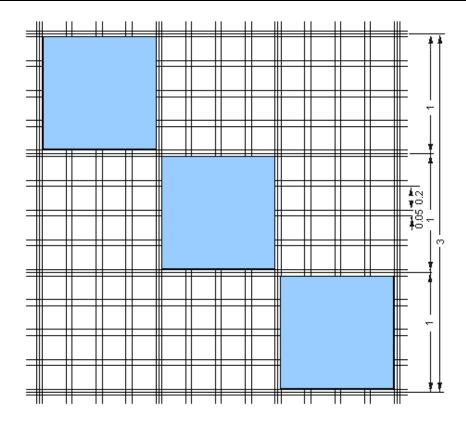
**Figure 1. Burker chamber.** One cell in one blue area means 1 x 10<sup>4</sup> cells/ml. (Source: <a href="http://openwetware.org/wiki/IGEM:University\_of\_Debrecen:\_transfection">http://openwetware.org/wiki/IGEM:University\_of\_Debrecen:\_transfection</a>)
