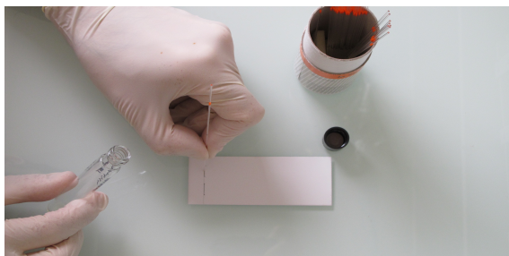
Figure 1. Loading the lipid samples with a capillary tube directly at the origin of the TLC plate
