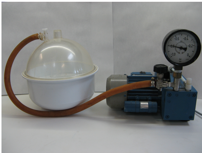
Figure 1. Vacuum jar and vacuum pump used for tissue infiltration
