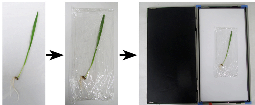
Figure 2. Setup of the radiolabeled sample on an imaging plate
