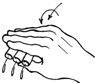
Figure 7. Hand-decanting supernatant from centrifuged ICS tubes
