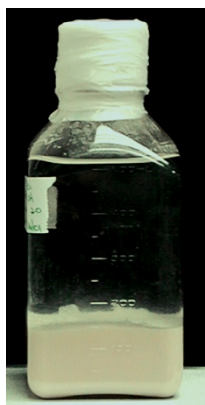
Figure 3. Ascaris embryos. Keep Ascaris embryos in 5 volume of ice-cold PBS, pH 2.0. Store at 4 °C.
